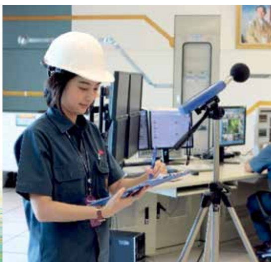
Noise level monitoring in the powerplant
